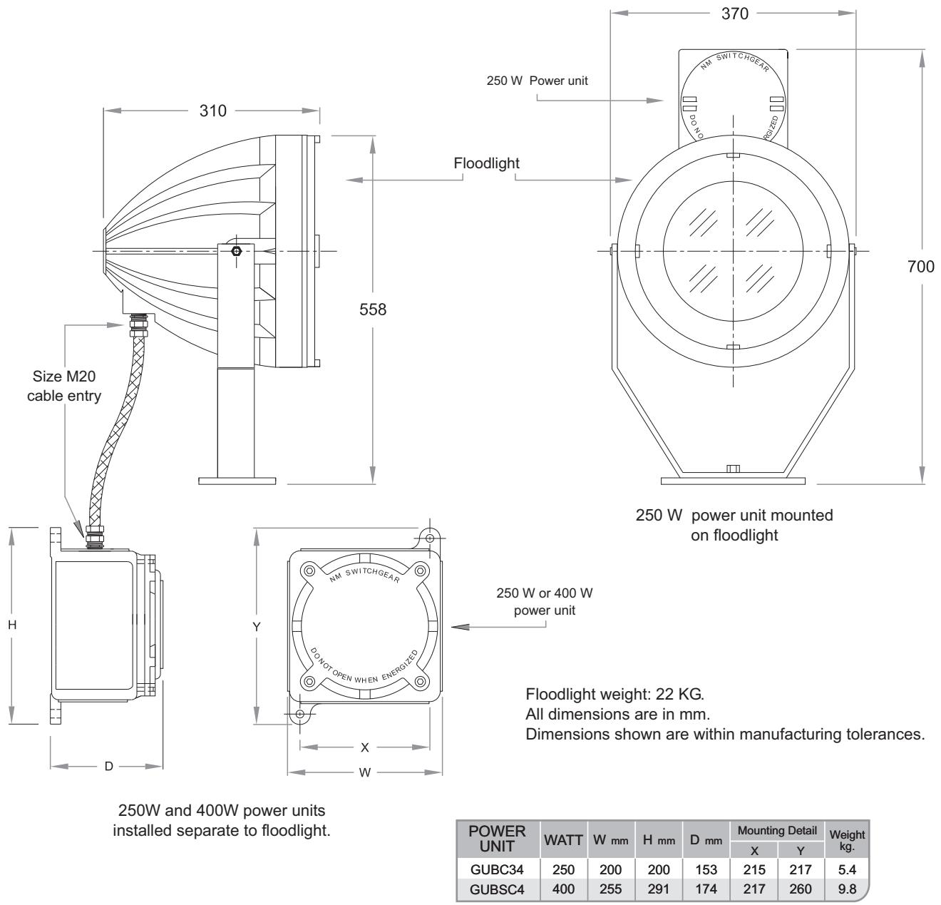
Both 250 and 400 watt floodlights have the same construction and dimensions as shown.
